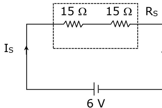
Effective resistance of the circuit,  $R_s = R_1 + R_2$
