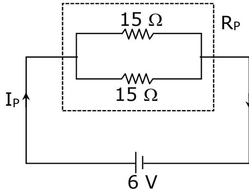
Effective resistance of the circuit,  $\frac{1}{R_p} = \frac{1}{R_1} + \frac{1}{R_2}$
